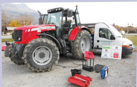
PASSAGE D'UN TRACTEUR AU BANC D'ESSAI MOTEUR
